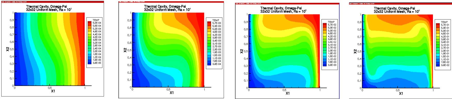
Norm equalization, “best mesh solutions,  $M = 32^2$  meshes,  $Ra = 10^6$
